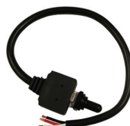
Weather Resistant Momentary SPDT Switch Controls two single wire circuits, permitting only one circuit to be energized at a time. Switch has a special rubber coated casing to resist moisture. Weather resistant boot included. 24V @ 15A / 12V @ 25A Mom On-Off-Mom On
