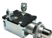
Momentary Push Button/Starter Switch 12V @ 15A / 6V @ 25A 5/8" Mount Hole Mom On-Off
