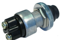
Heavy Duty Push Button/Horn Dust and moisture resistant boot. 12V @ 60A/ 24V @ 40A 5/8" Mount Hole Mom On-Off
