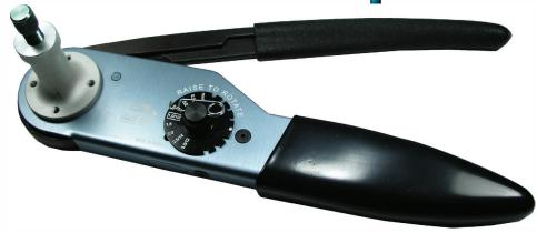
This solid barrel crimping tool has eight indent hand crimps for 12-20AWG Solid Contacts. It is compatible for DT, DTM, DTP, DTHD series and other Deutsch industrial connector families. For use with solid contacts only.
